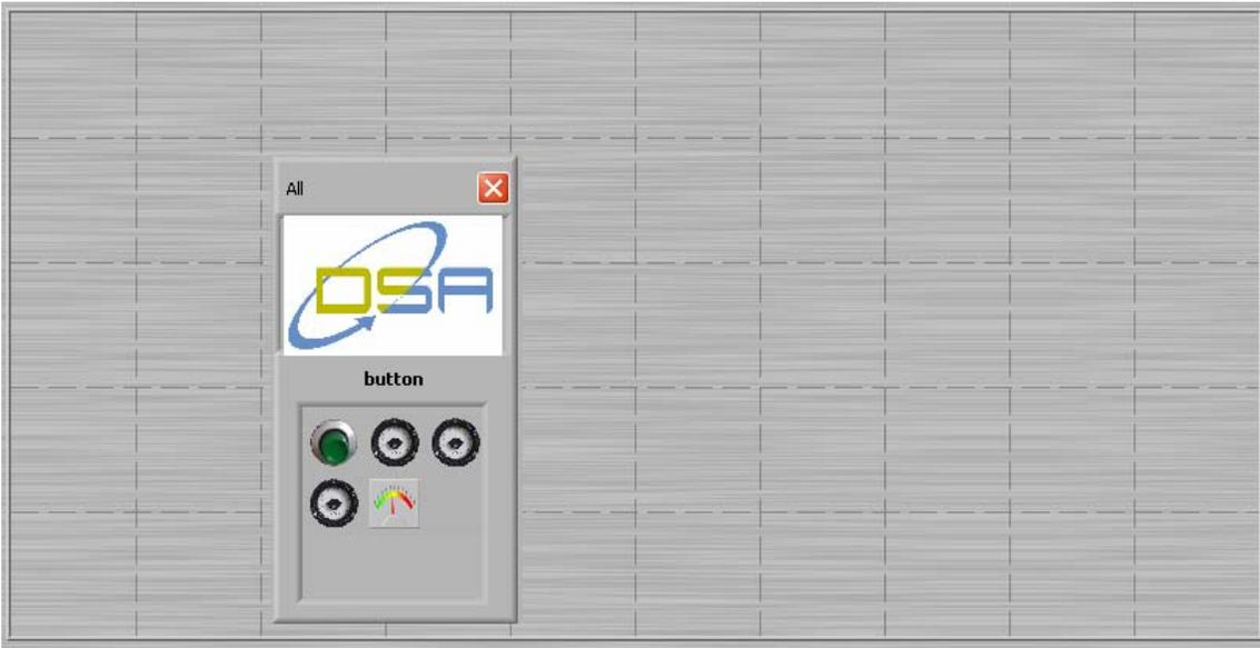
After selecting the desired control from the palette, the control panel designer clicks on a blank portion of the control panel area to identify where the application should place the control object. This
