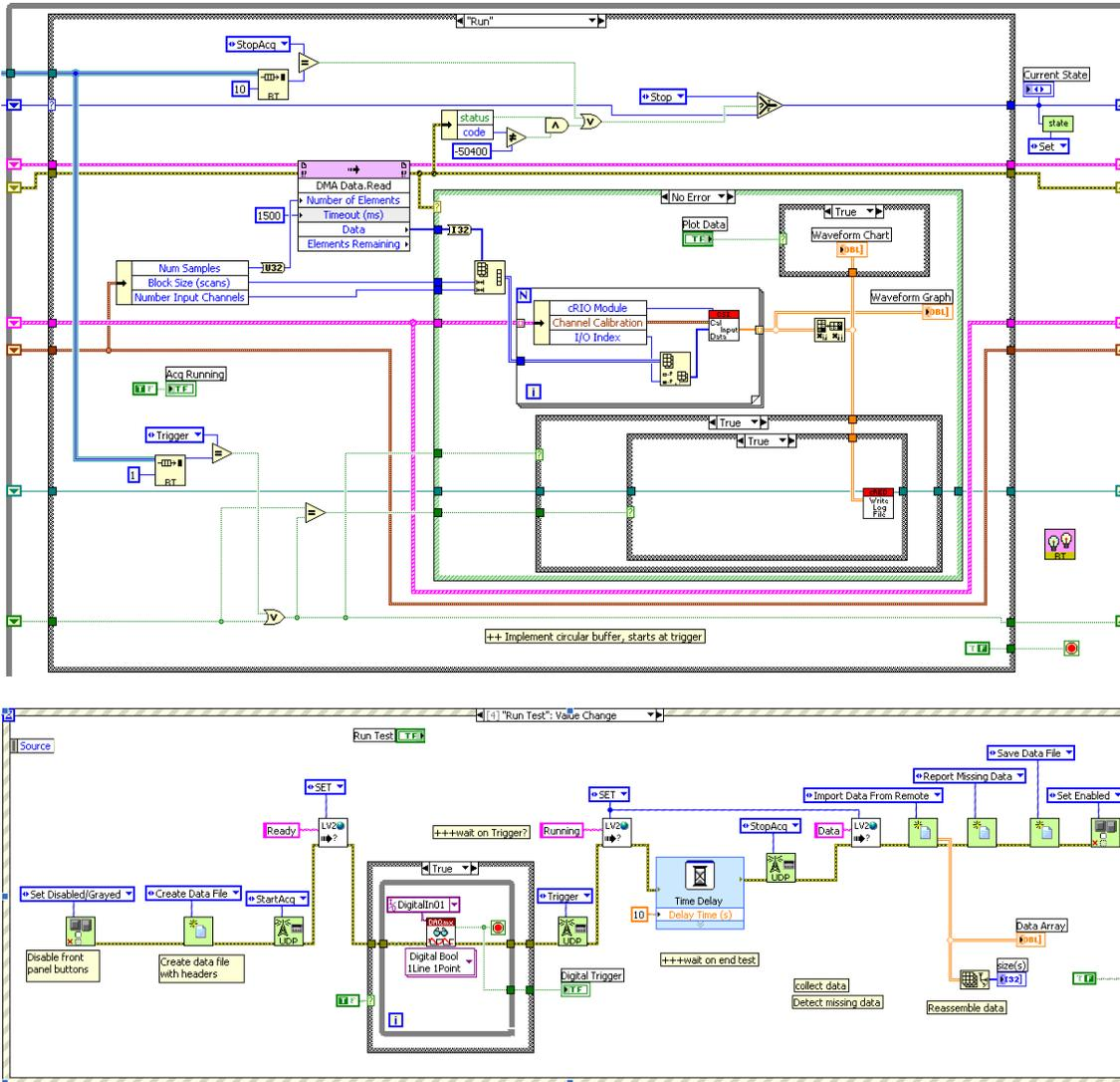
Figure 2 - The FPGA data gathering code on the remote cRIO system, along with the host PC UDP communication code
