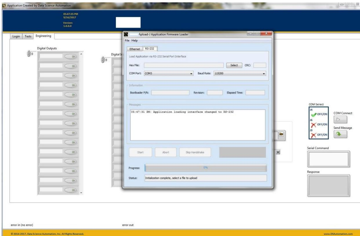
Figure 4 LabVIEW passing connection and hex file parameters to third party EXE
