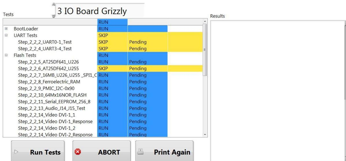
Figure 3 Operator Screen, with single step skipped and skipped group example
