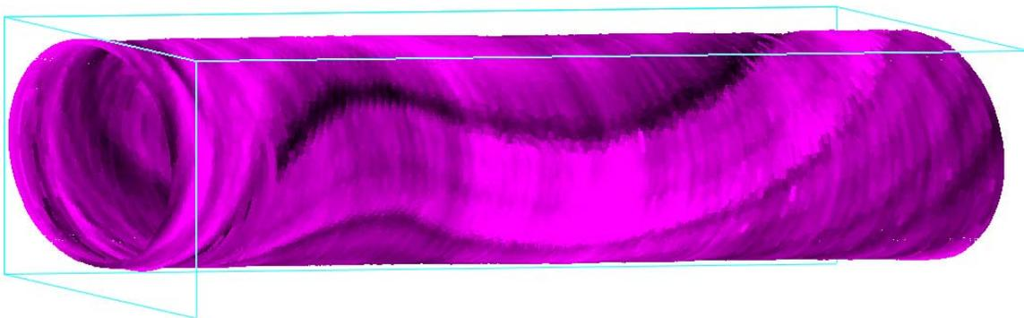
Figure 4. 3D Visualization of Circumferential and Axial Non-Uniformity of Wall Thickness
