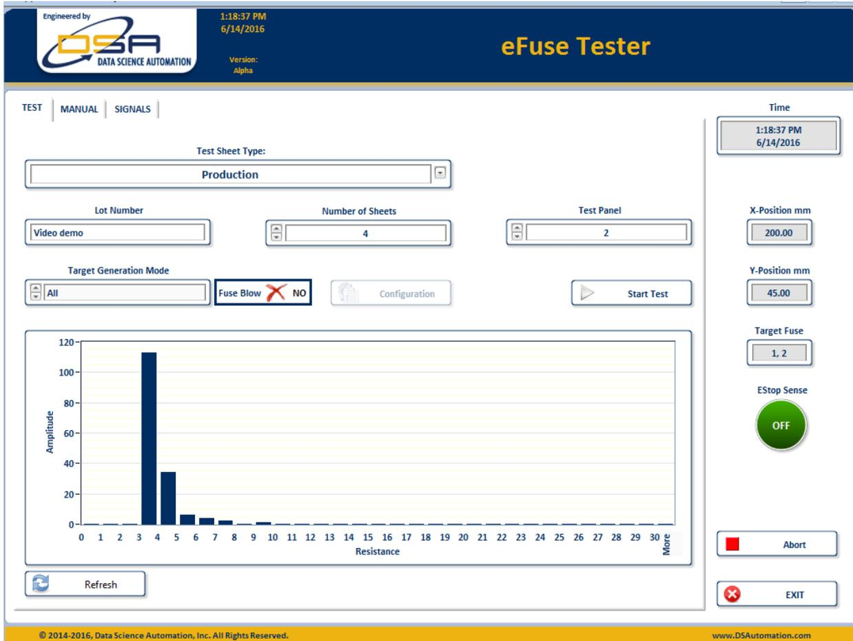
**Figure 1 Fuse resistances, binned by value to show variance of production. All higher values, and open circuits, are collected in the last bin**
