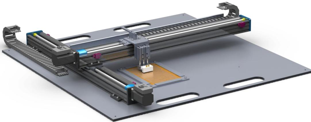
**Figure 2 Mechanical movement and end effector design.**
