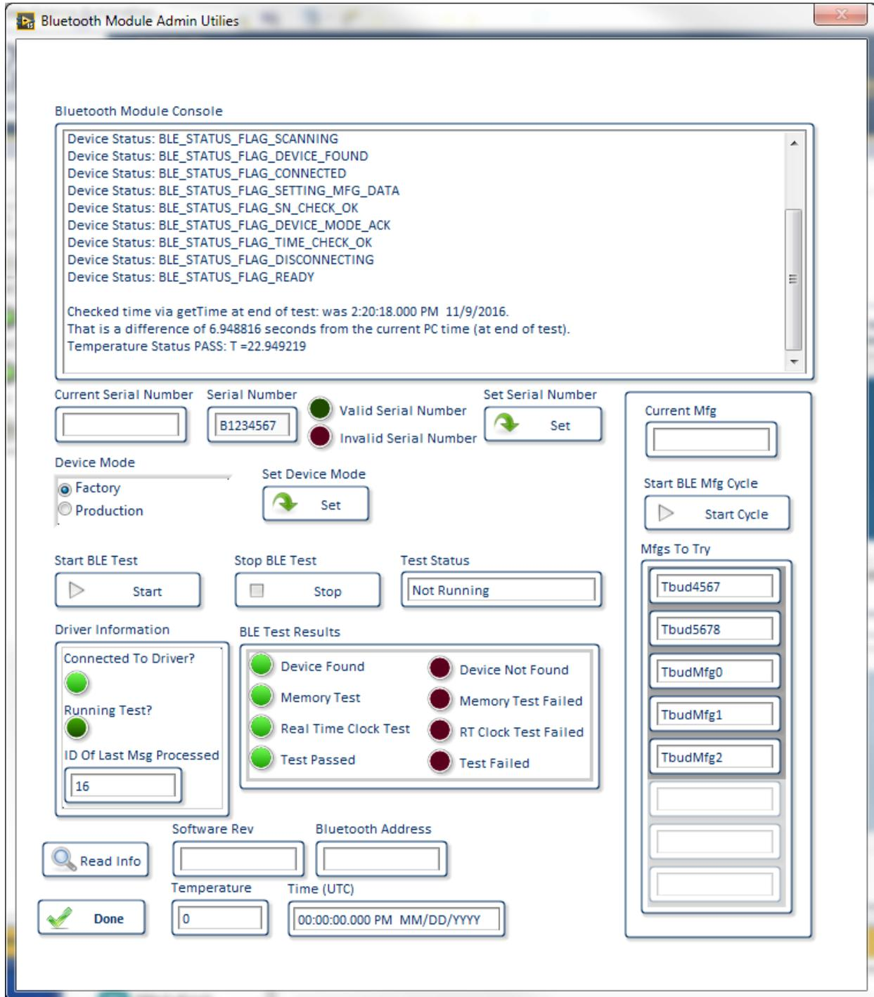
Figure 1 - Bluetooth communication screen, with messaging and test results per DUT
