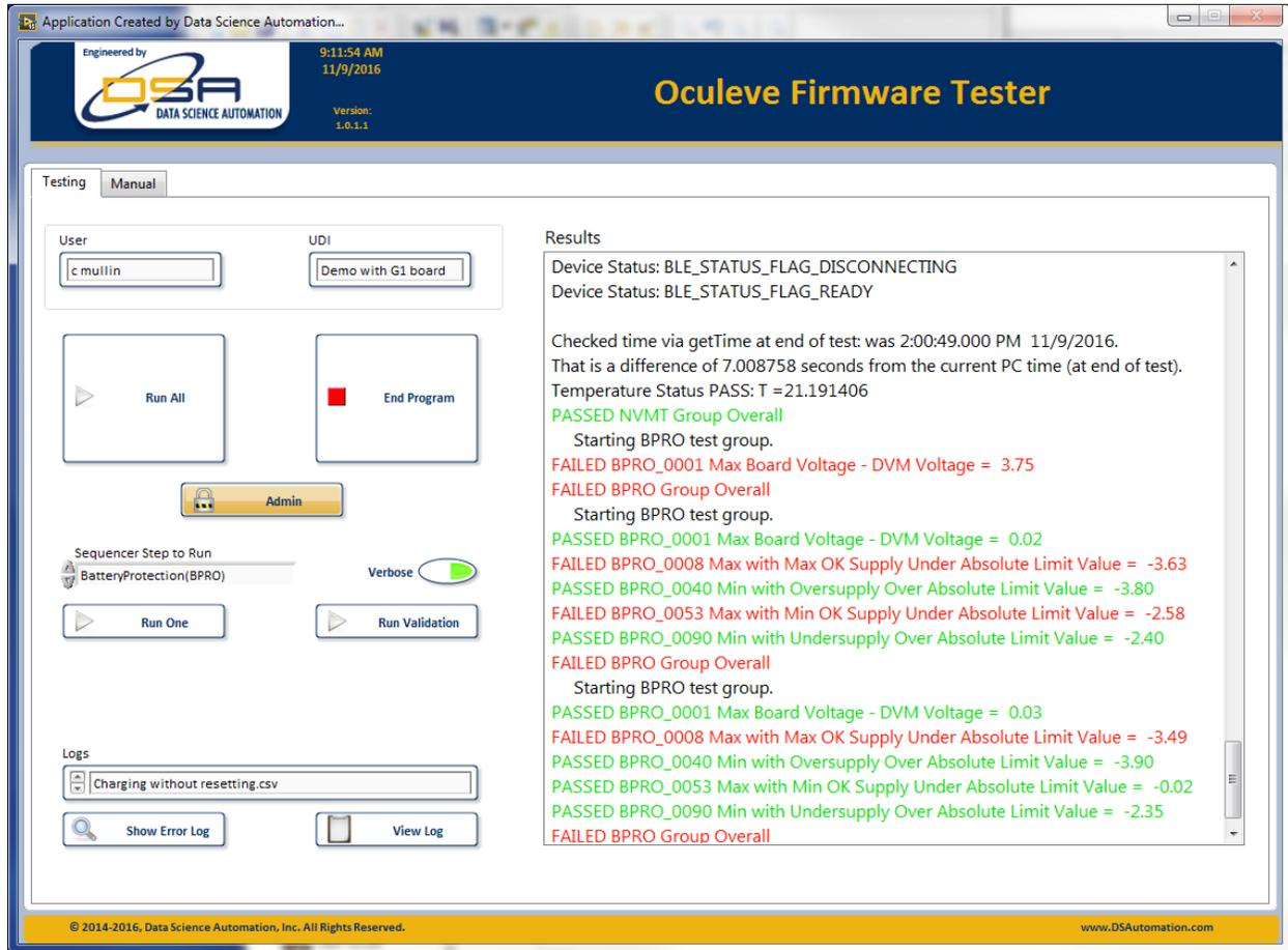
**Figure 2 - Example test result with known-bad board, indicating passing and failing steps, arranged by test group.**
