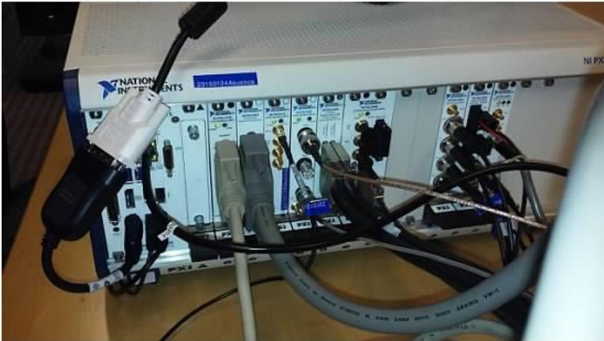
**Figure 1** A variety of modular instruments were used to characterize analog and digital microphones.
