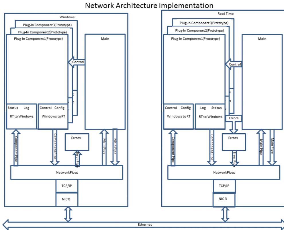
**Figure 1. Network architecture for test application written in LabVIEW**
