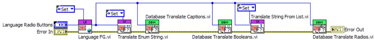
**Figure 1. A Portion of the Framework Used to Support the Localization Software.**
