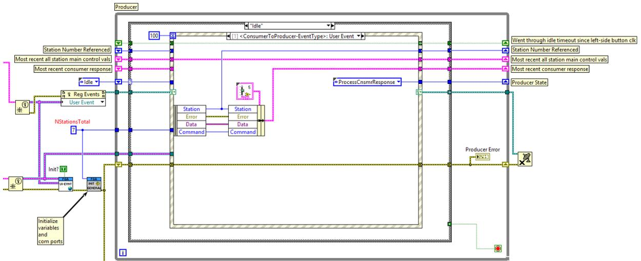
**Figure 1. Central State Machine for Automating Calibration and Tests for Gas Analyzers.**
