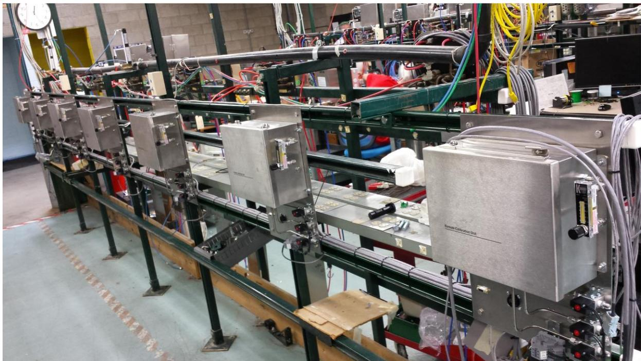
**Figure 2. Seven Calibration Units for Gas Analyzers, Automated by a Single LabVIEW Program on a PC (Not Shown).**
