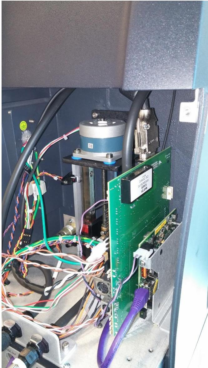
**Figure 3 – The Interior of the TGA Features an NI-9606 That Brings the Product to Life.**
