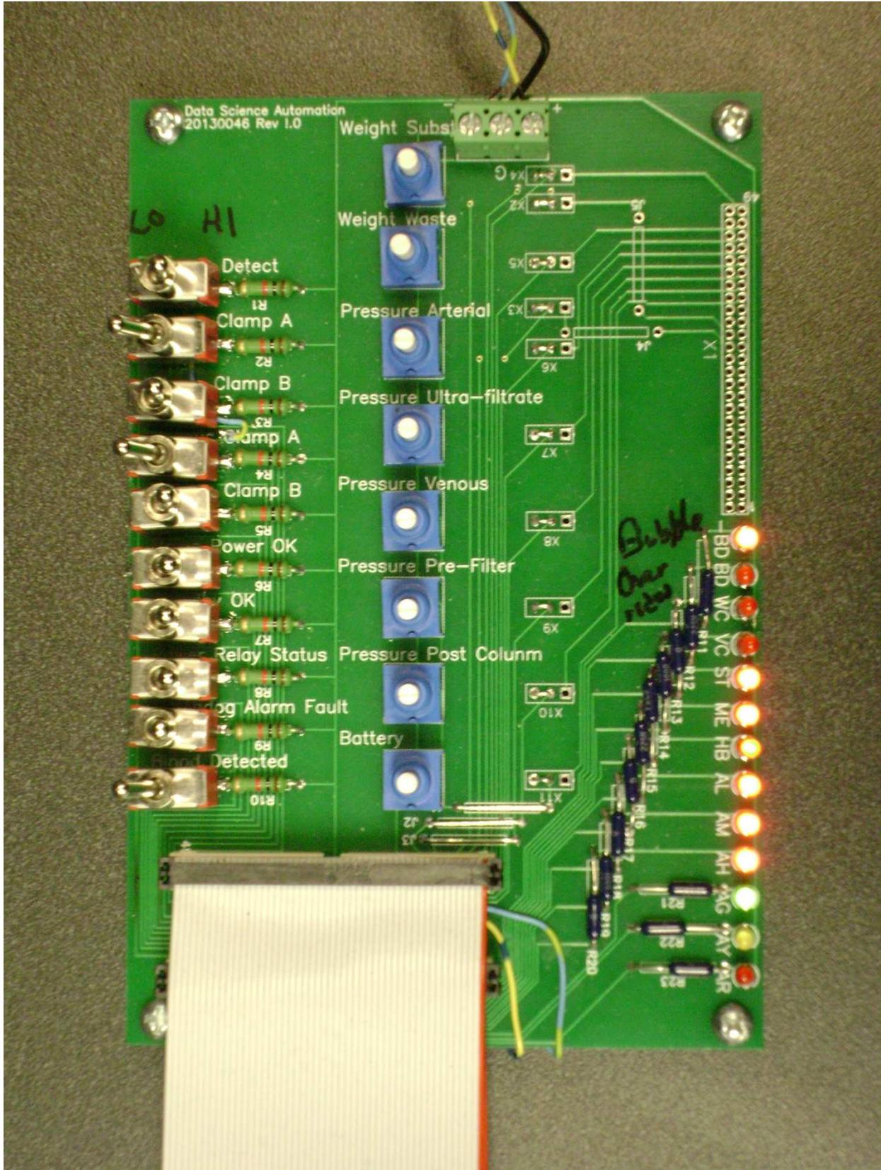
**Figure 1 - Photograph of the Hardware Simulator Board**
