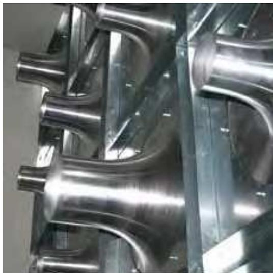
**Figure 2. Typical Calibrated Nozzles used to Determine Air Flow Rate (CFM)**
