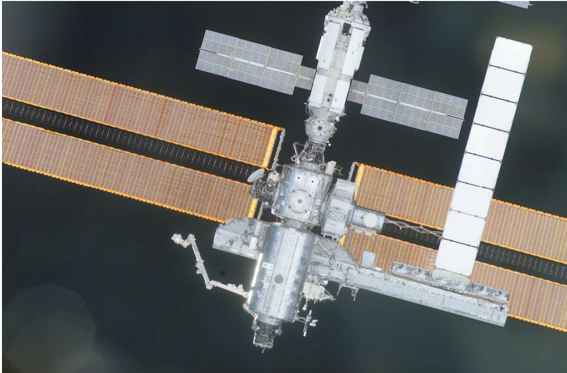
Figure 1. Satellites contain both solar power panels and radiator panels
