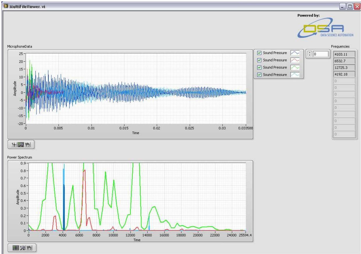
Figure 3 - Comparison of Known Good to Known Bad Gold Bars Through Use of TDMS Files
