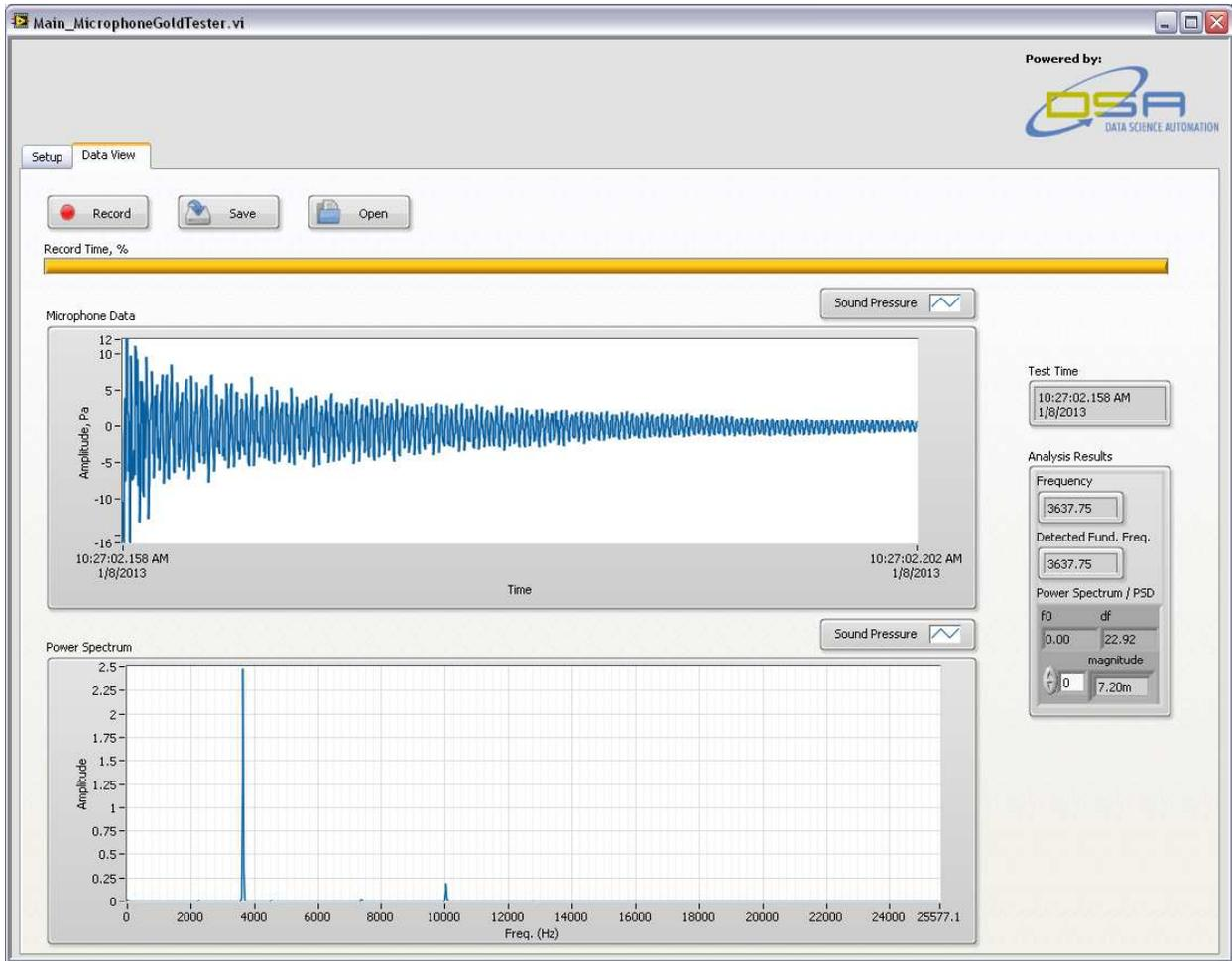
Figure 2 - Counterfeit Bar - No Extended Ringing and Frequency Detected Below 4100Hz
