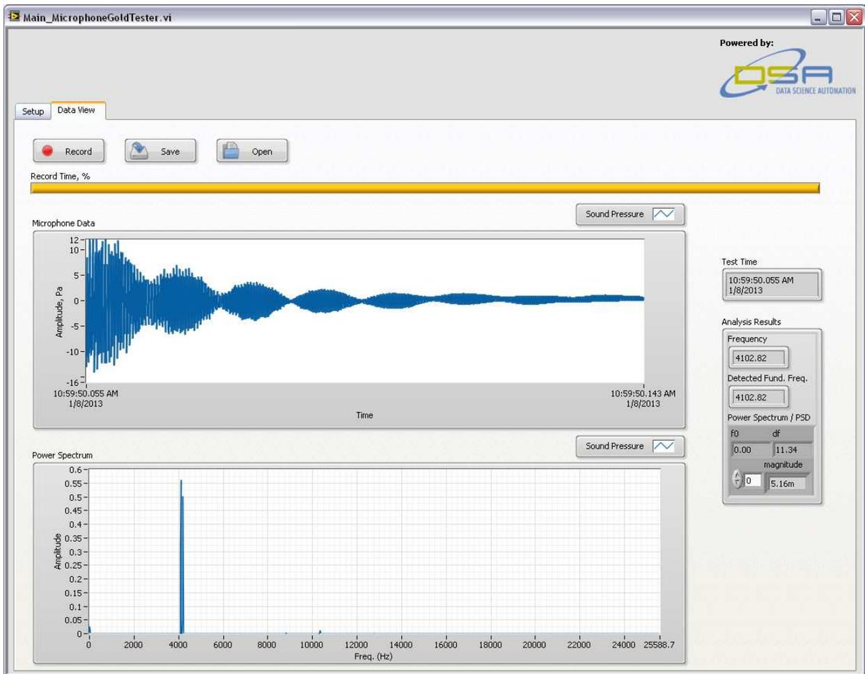
**Figure 1 - Known Good Gold Bar - Ringing Evident with Strong Frequency component at ~4100Hz**
