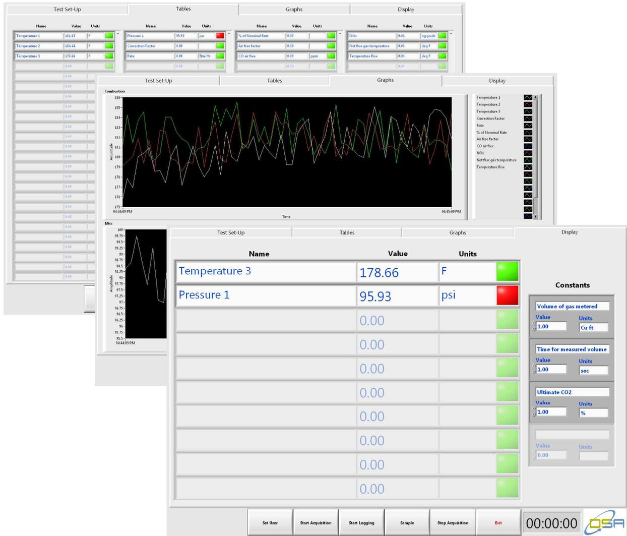
**Figure 2 - Tabs allow the user to view the same data in different ways depending on the situation; for example, a large display allows the user to see important data from across a room.**
