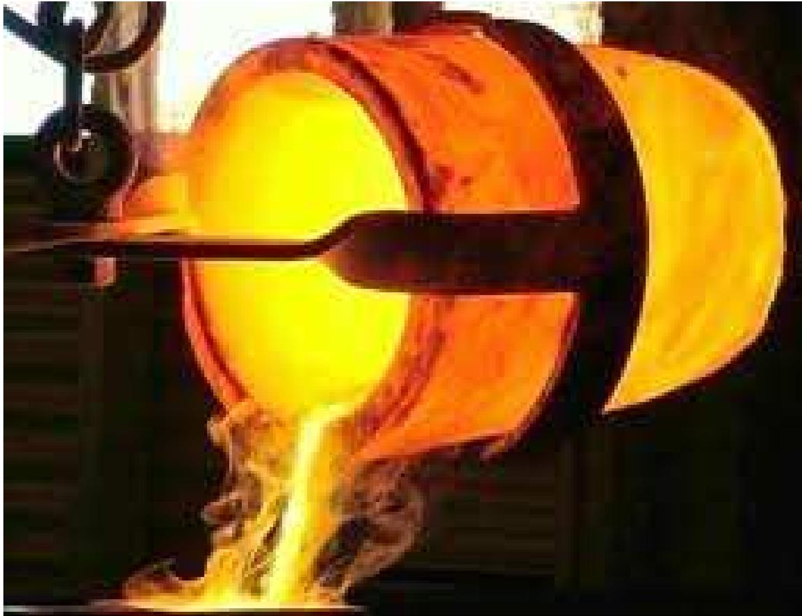
**Figure 1 - Molten metal being poured out of a crucible into a mold for casting.**
