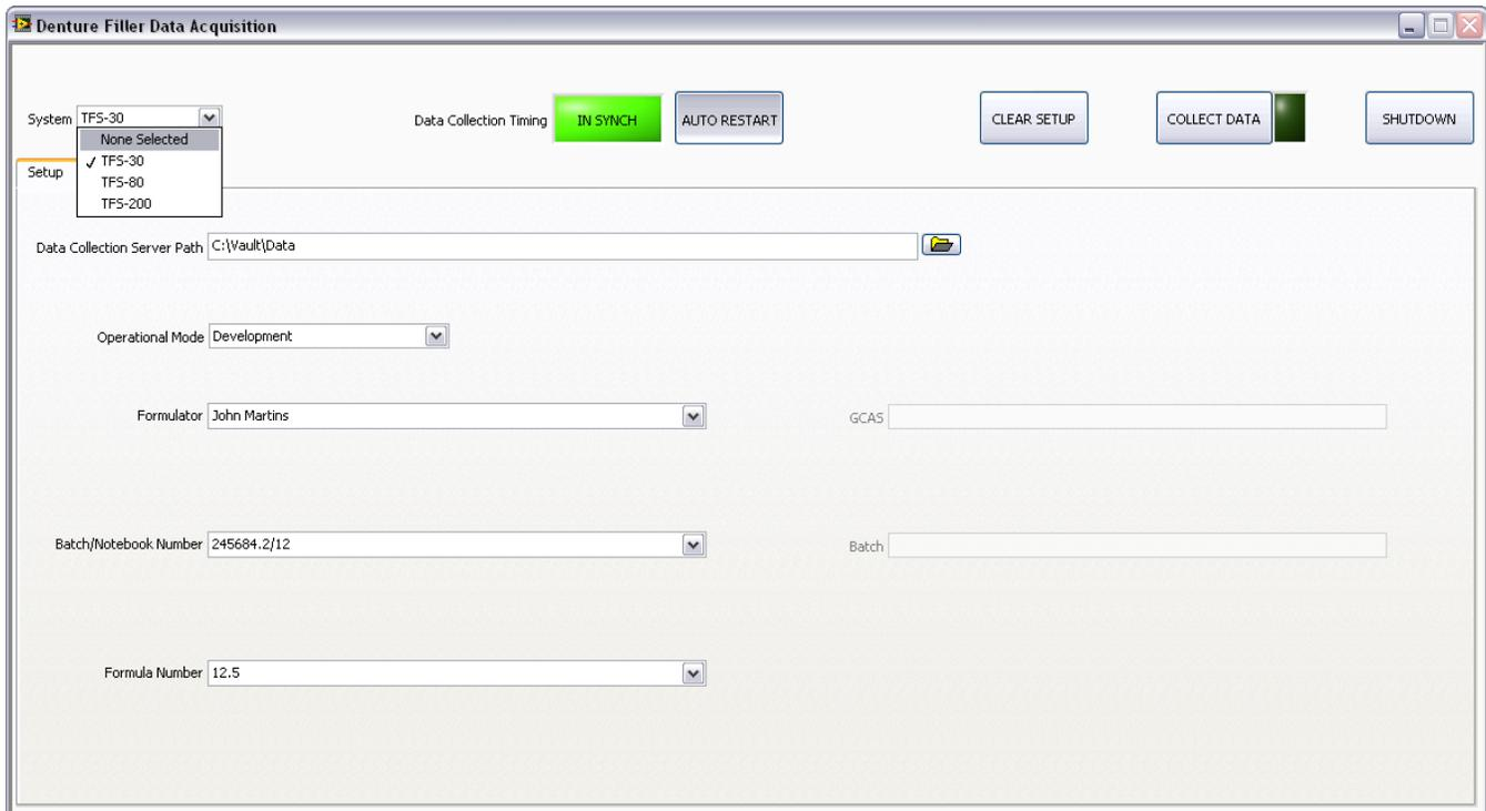
Figure 1 - Configuration Screen. This is where the operator selects database provided lists of Formulators, Batches, and Formula Numbers that the system is going to be used to test.
