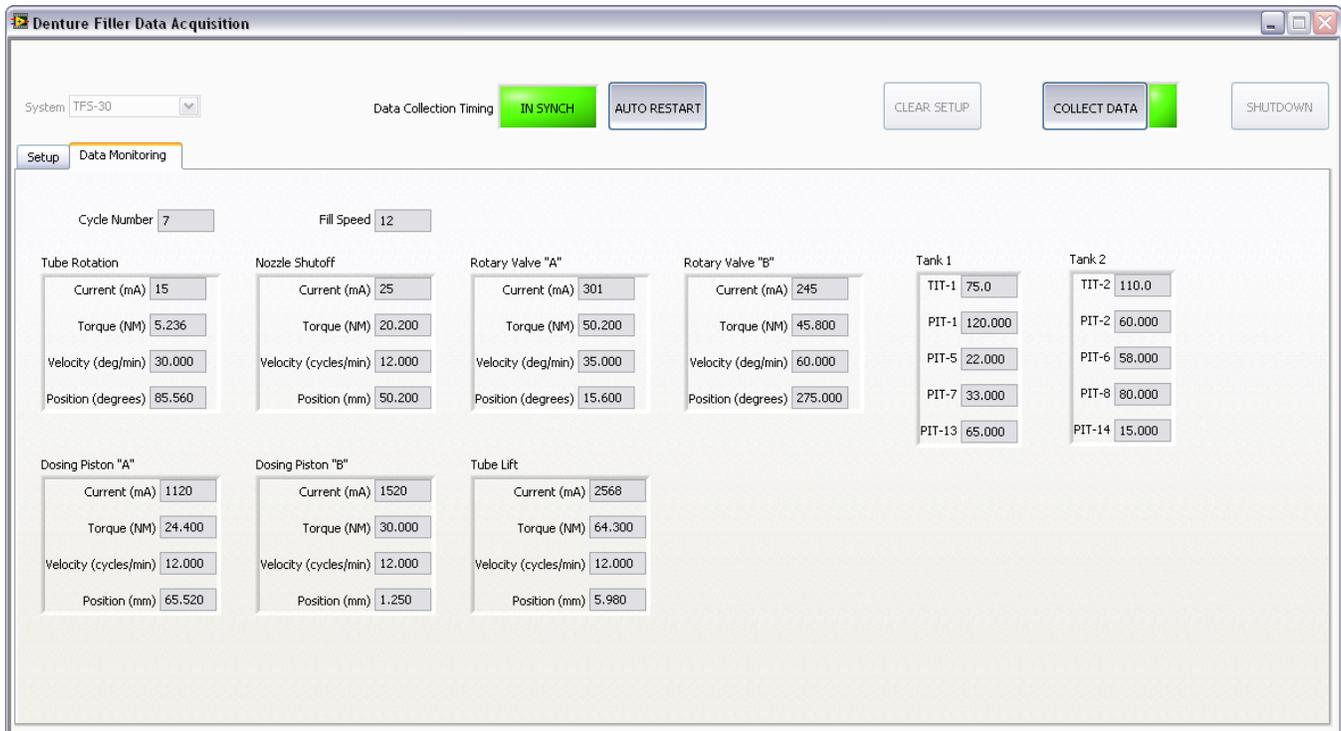
Figure 2 – Data Monitoring Screen. This screen provides live data to the operator while the system is up and running, regardless of whether data collection is set to record to file.
