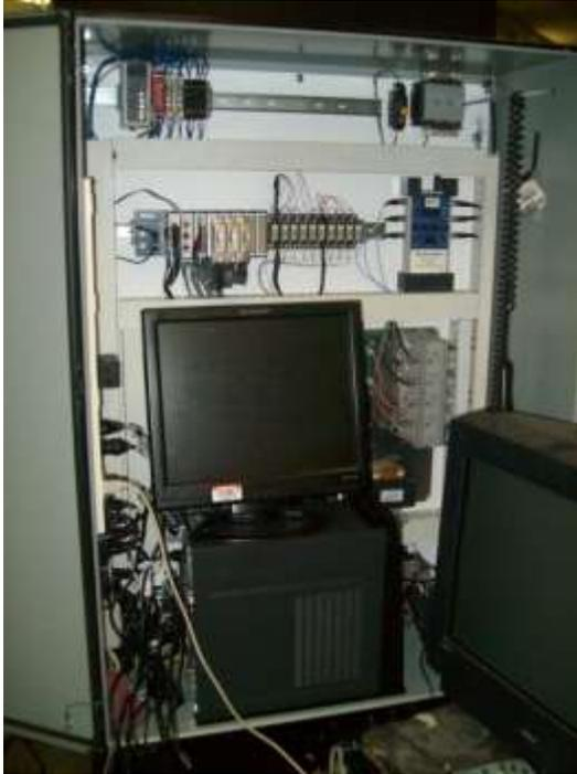
**Figure 3. Test station rear view shows fully populated Compact DAQ Chassis**
