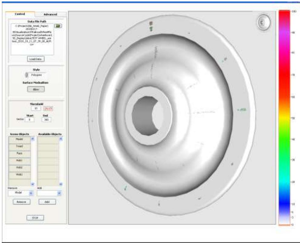
Figure 1. 3D-Scan maps C-Scan data onto a model of the DUT.
