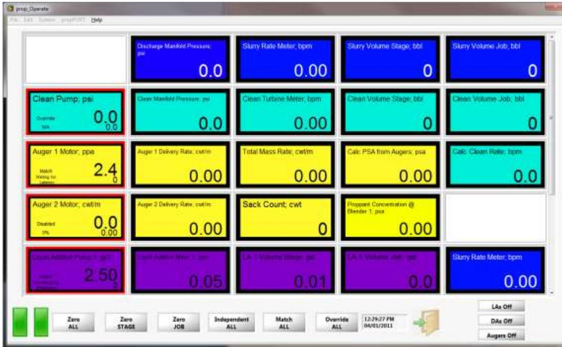
**Figure 2**–This screen is the operate screen that allows the operator to set up and display the data that is desired for the job.
