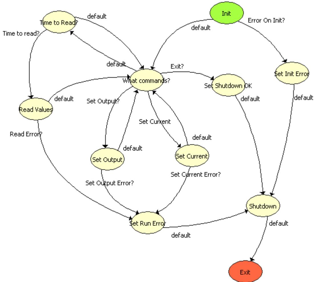
**Figure 4. Manual Mode State Diagram. In manual mode, the state of the load is periodically checked. When new commands are received from the User Interface, they are executed.**
