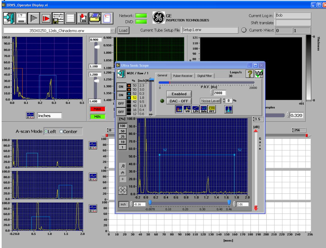
Figure 1 Operator GUI, including parallel displays, logging charts and pop-up central core functions, all shown in real-time
