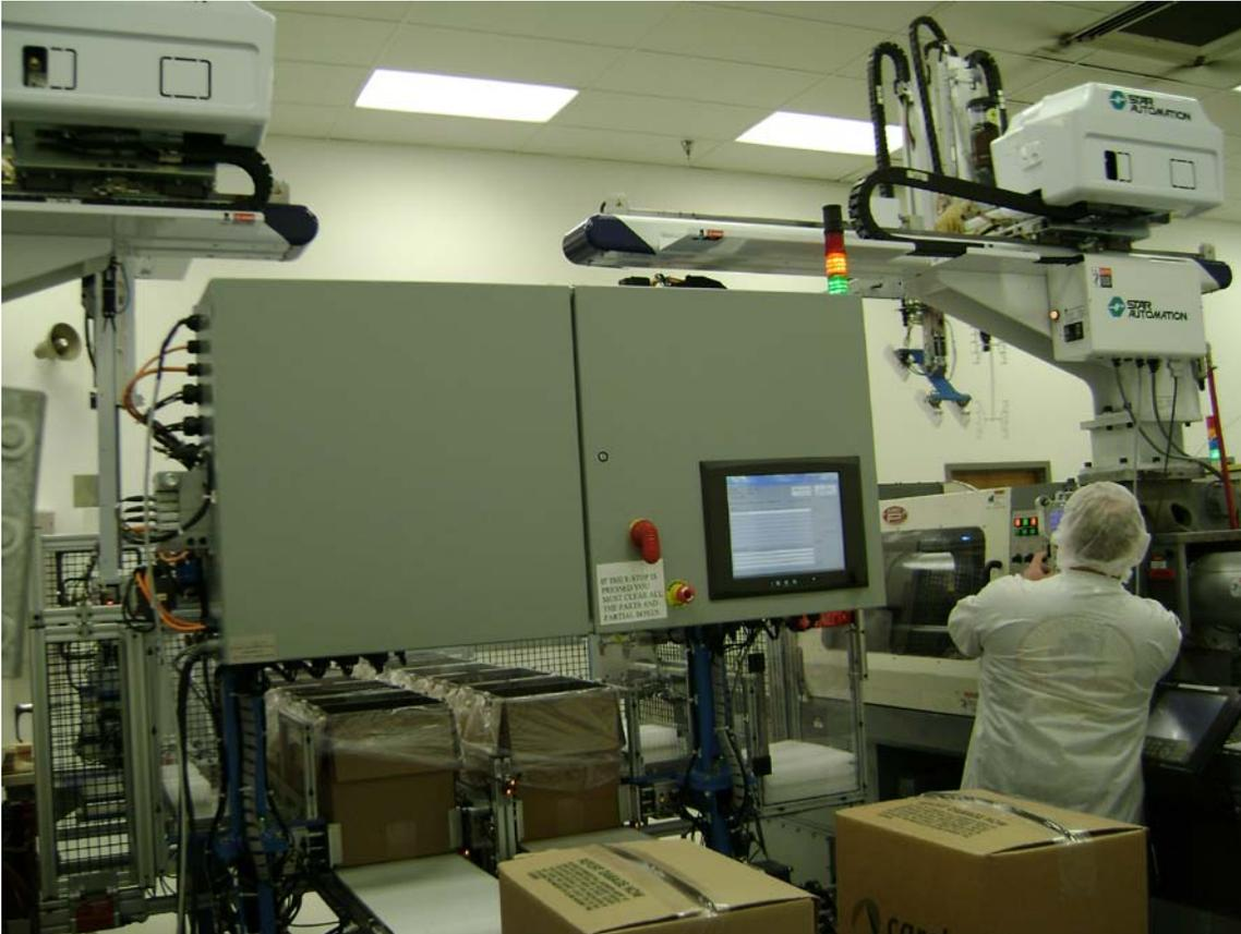
**Figure 2 – The main packaging machine communicates with and receives parts from two asynchronously running Star Automation robots which remove parts from the injection molding machines.**
