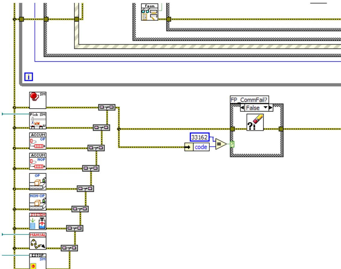
**Figure 1 – Main Block Diagram shows the nine separate subsystem state machines that all run in parallel to make the packaging machine work.**
