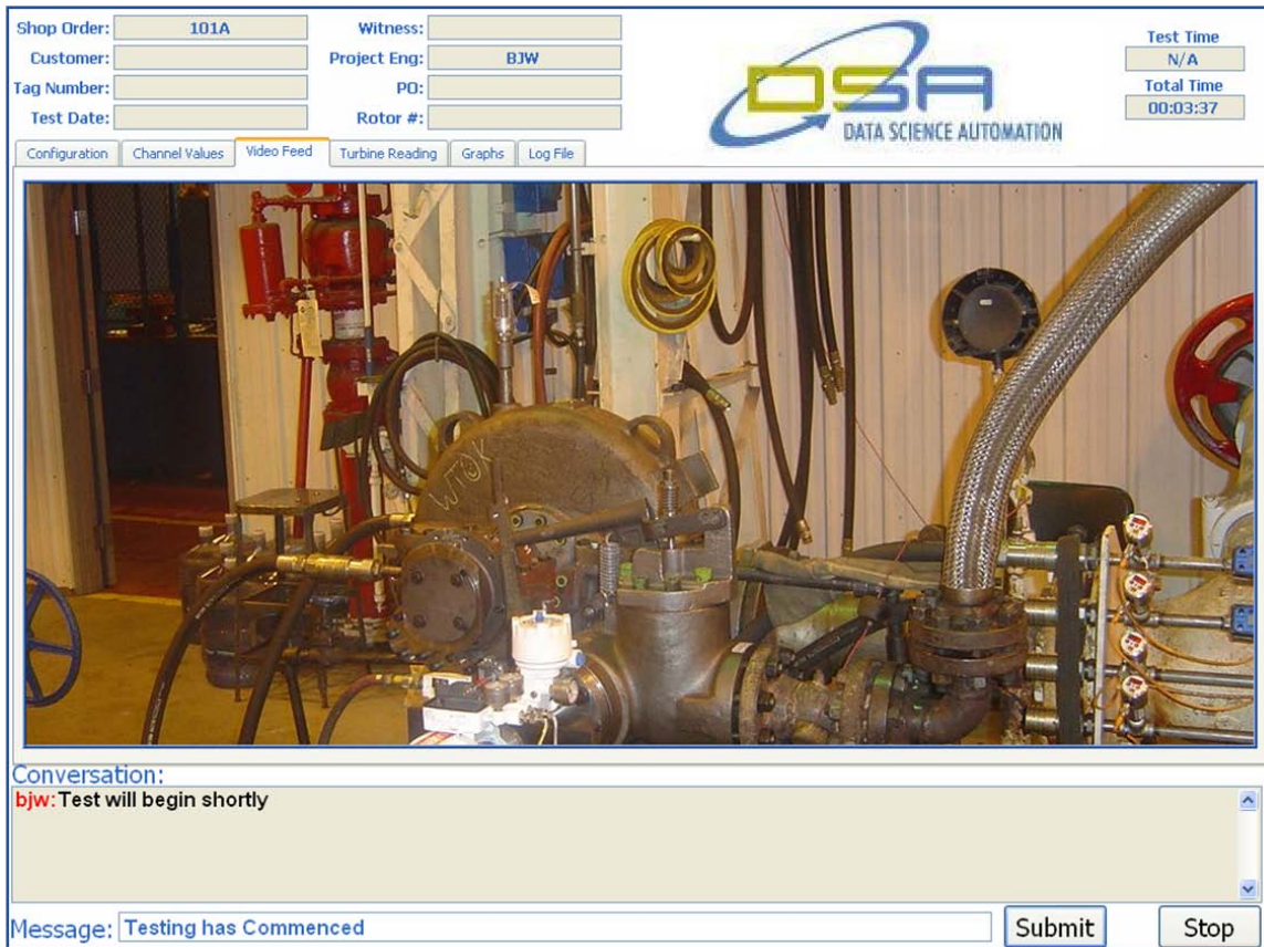
Figure 2 – This screen show live video of a test in progress, along with the chat window that supports real-time communications between the test operator and multiple remote witnesses.
