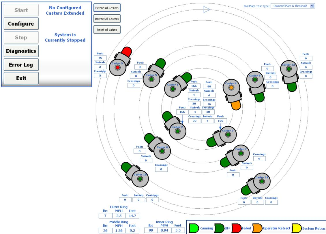
Figure 1 – Color coding in the user interface allows the operator to see at a glance the status of the casters currently under test.
