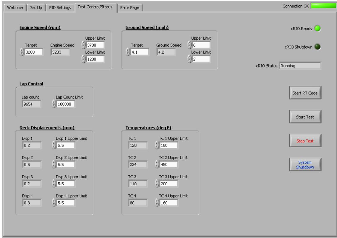
Figure 2 – Windows Host Program - Test Control/Status Tab
