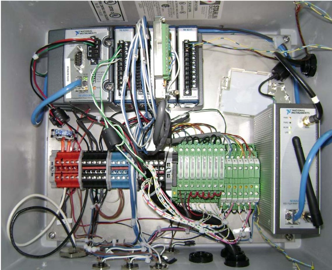
Figure 1 – cRIO Control System with WAP-3701 for 802.11g Wireless Communication (during assembly)
