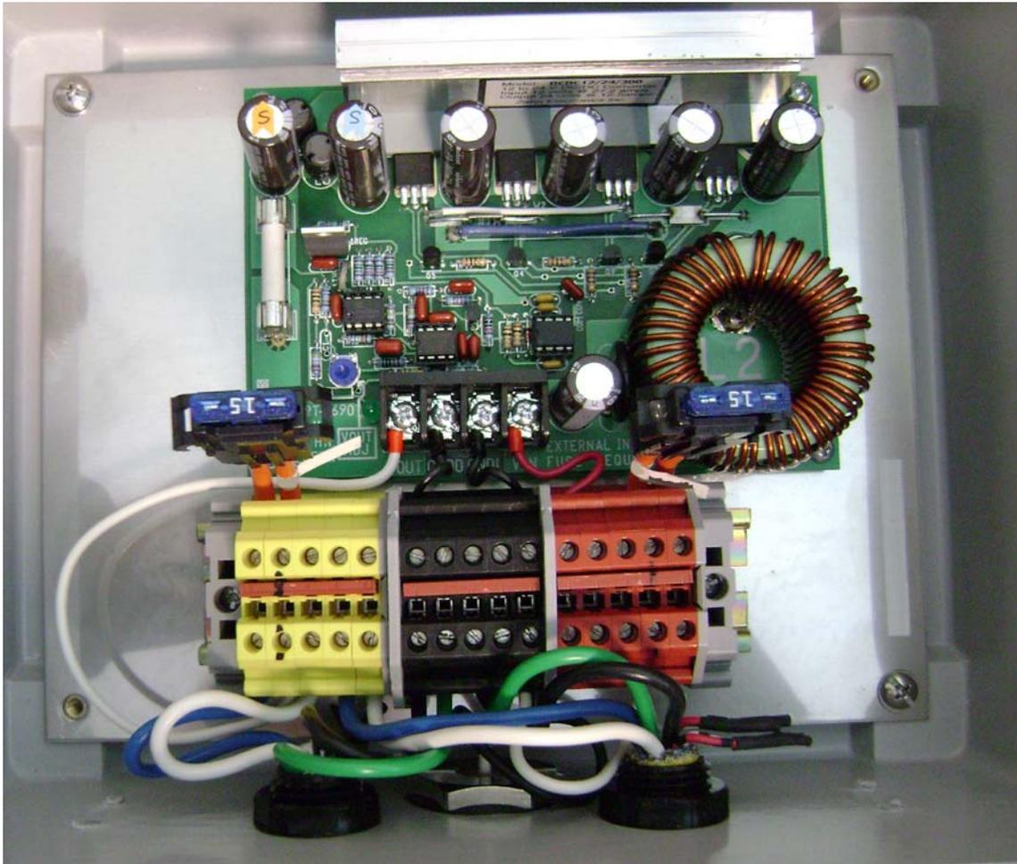
Figure X – 12V to 24V Step Up Converter from Zahn Electronics
