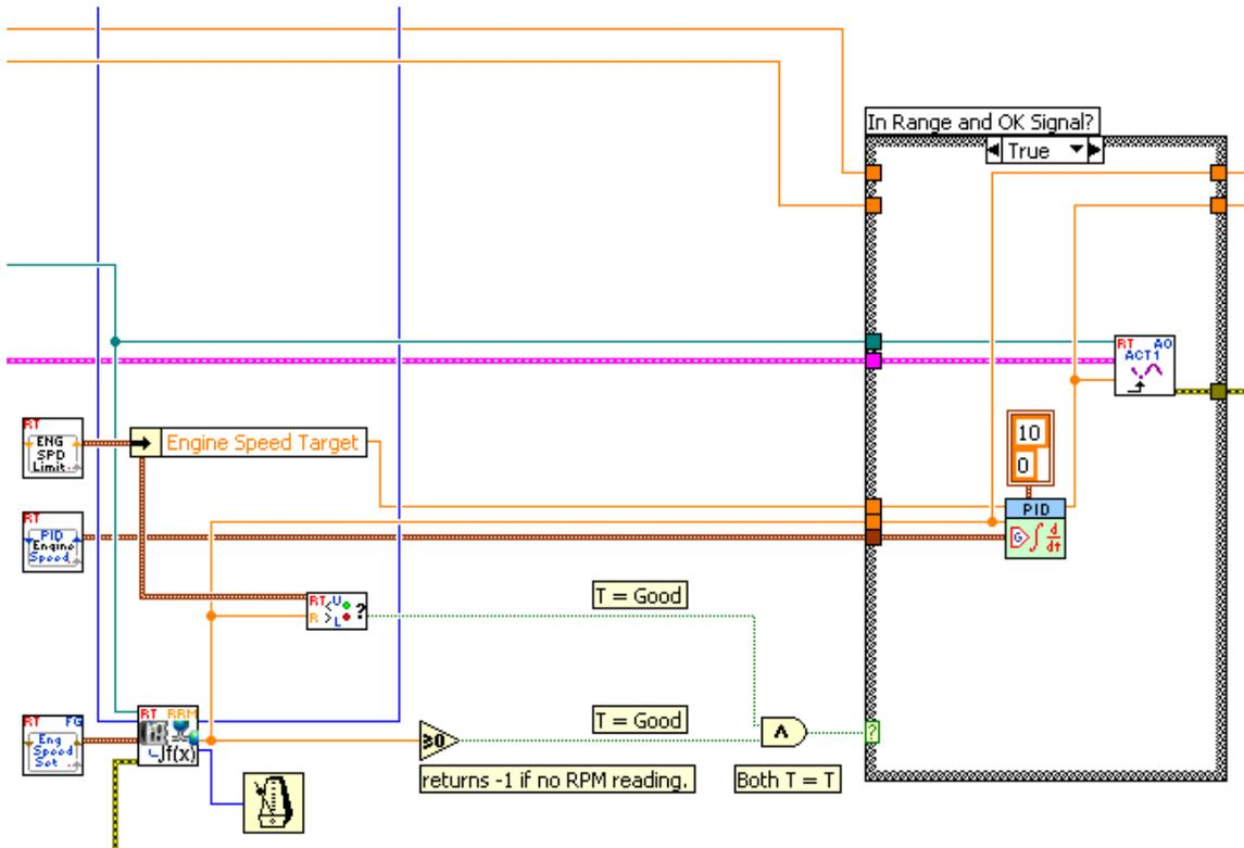
Figure X – Engine Speed PID Case of State Machine
