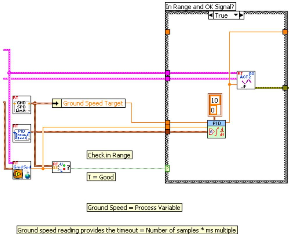
Figure X – Ground Speed PID Control Loop Code
