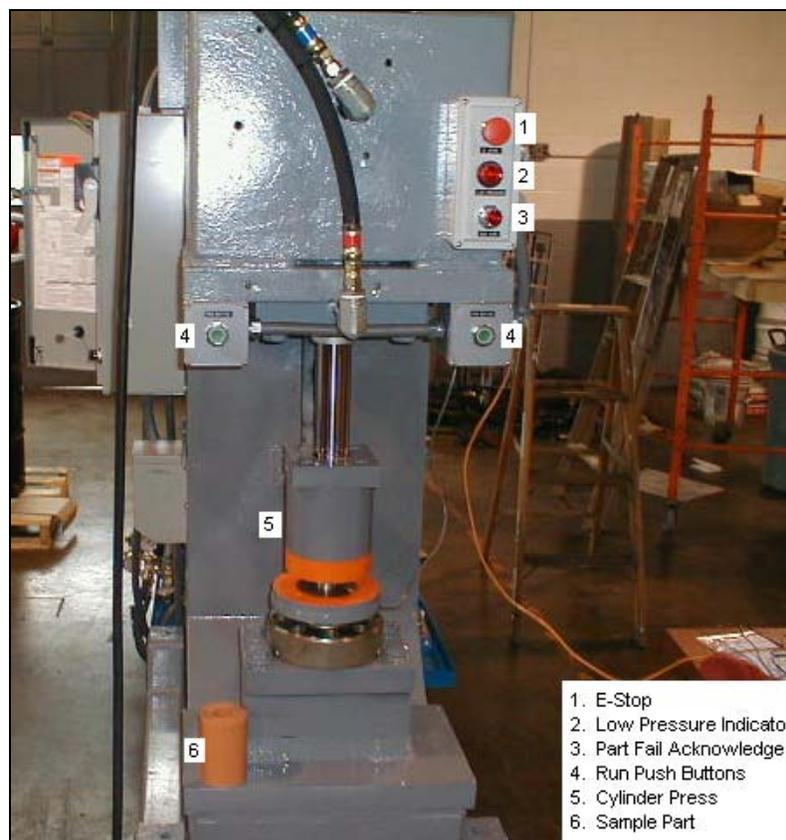
**Figure 2. Hydraulic Load Frame and Operator Controls**
