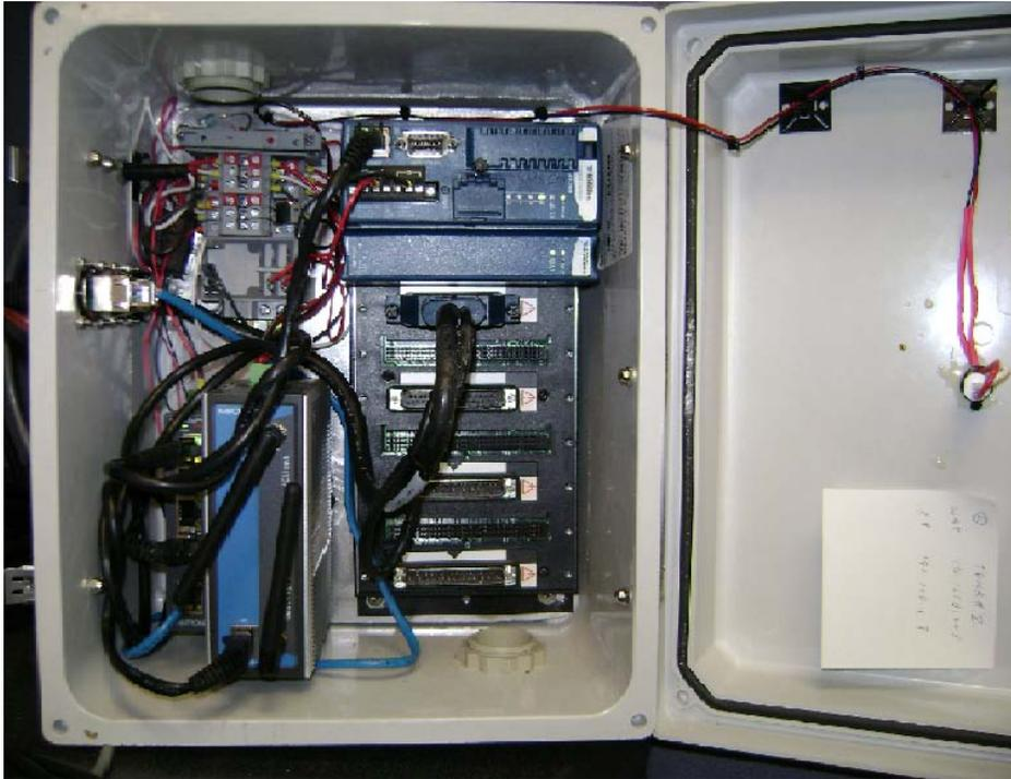
Figure 1 – This is a picture of the inside a truck mounted DAQ unit.
