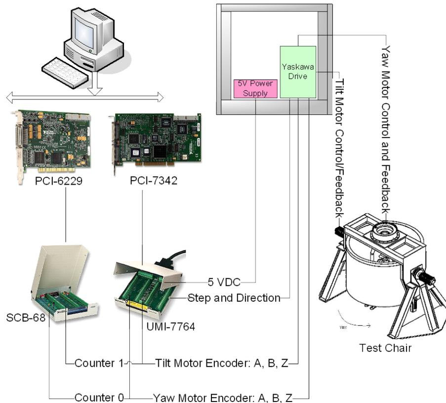
**Figure 1. Neuro-Otologic Test System**
