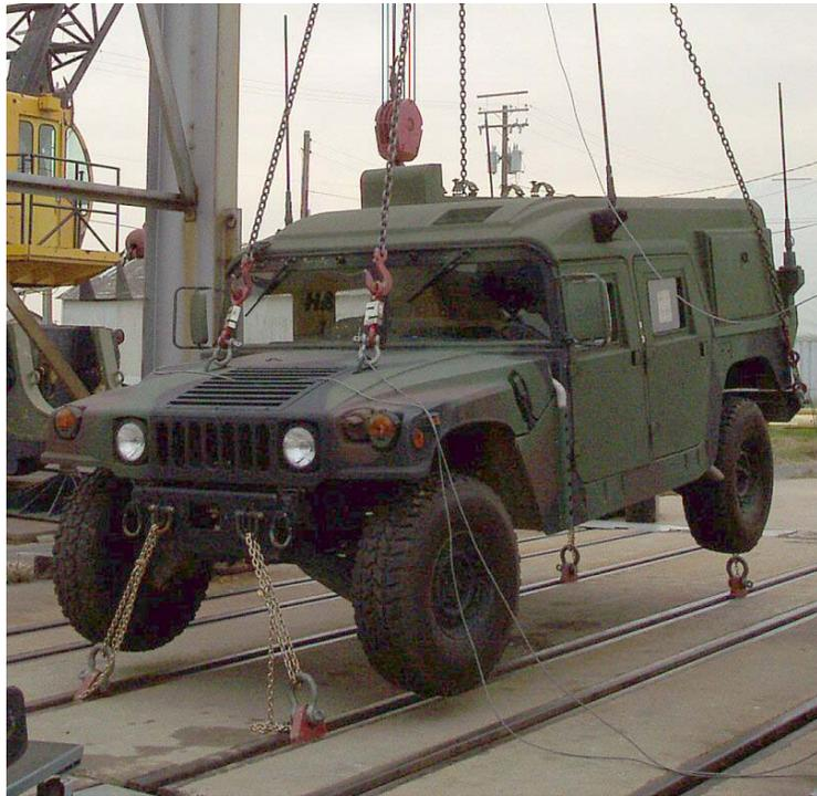
Figure 1. 1-G Lift Test
