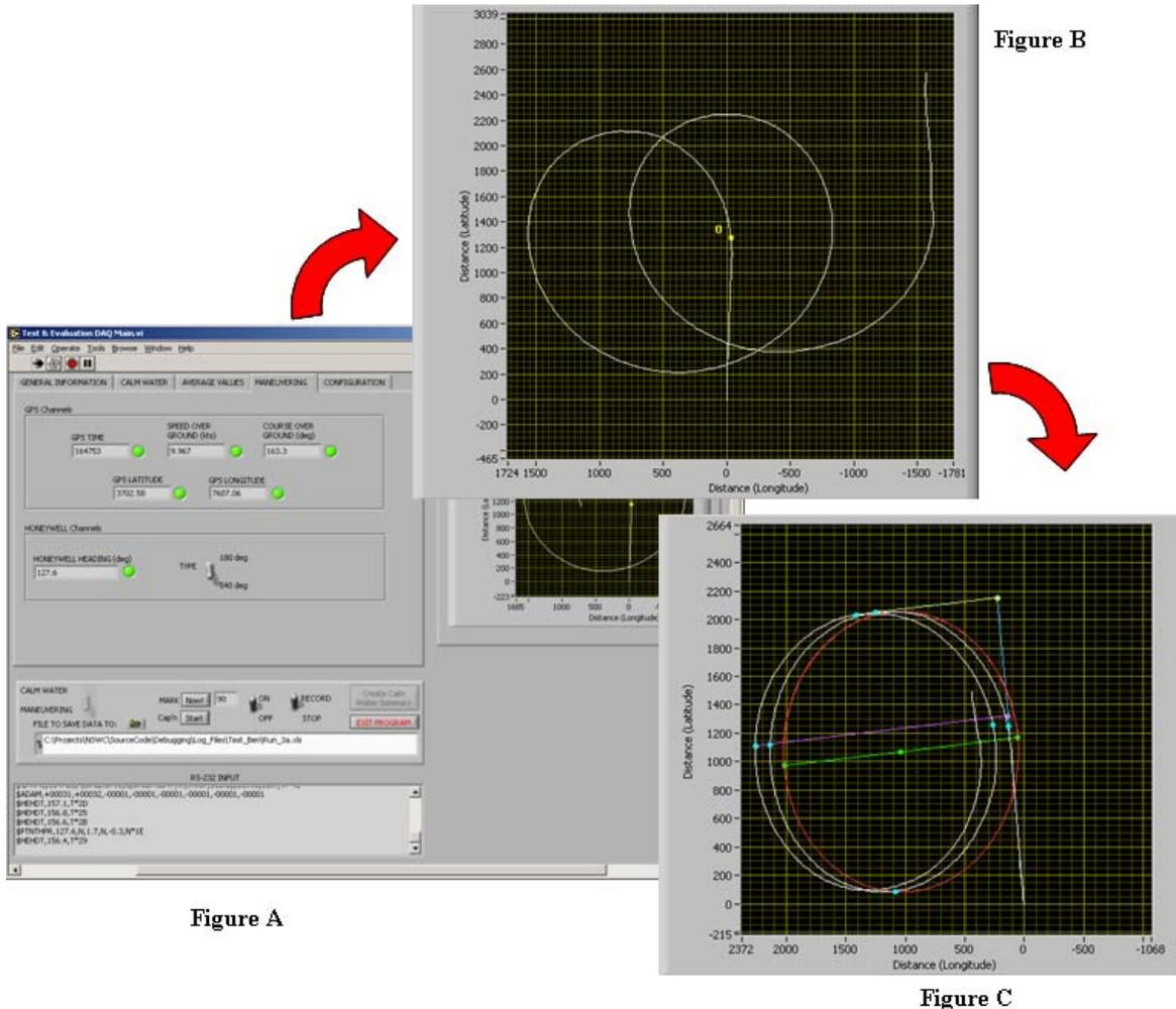
Figure 2. Determining Tactical Diameter, A) User Interface, B) Raw Track (Pretzel), and C) Corrected Plot
