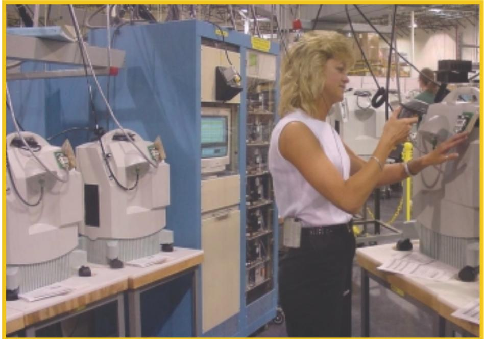
*A wireless barcode scanner and battery-operated belt receiver allows an operator to move anywhere along the test line, adding, removing, and checking on UUTs.*
