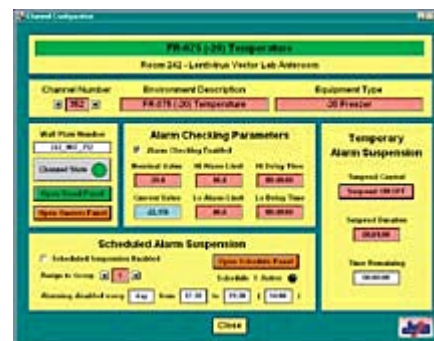
Figure 1: Panel for configuring the parameters of an individual data acquisition channel
